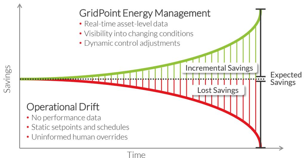
Figure 1. Operational drift causes buildings to gradually stray from expected savings over time but GridPoint's energy management system provides the data to recoup and exceed those savings.
